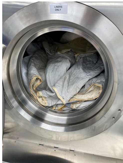
Figure 6 - Samples in garment bags mixed with liners for ballast.
