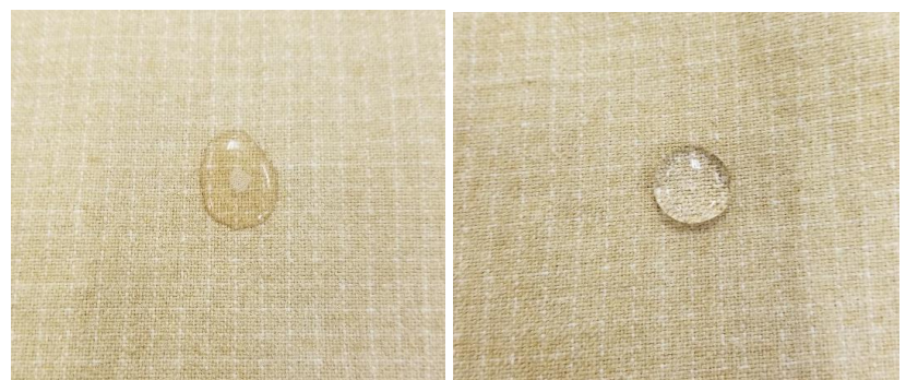
Figure 2 - Appearance of Applied Water Droplets on Outer Shell Sample; Before any cleaning – left, After 30 Cleaning Cycles - right
