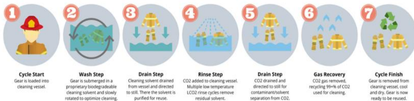
Figure 1 – CO 2 + Cleaning Process
