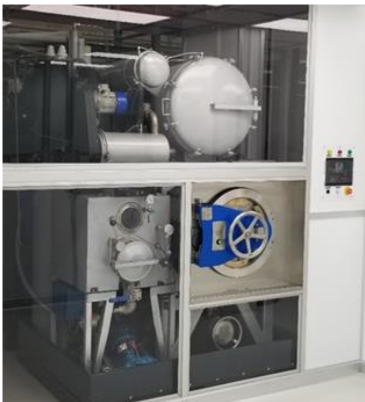
Figure 1 – CO 2 + FireFighter Gear Cleaning System – Emergency Technical Decon – Eagan, MN
