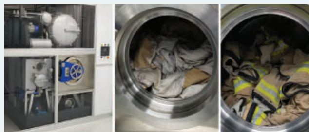
Figure E1. LCO 2 Cleaning System in Emergency Technical Decon Facility, Eagan, MN, Processing Facility (left); Liners (center); and Outer Shells (right) Inside Cleaning Vessel
