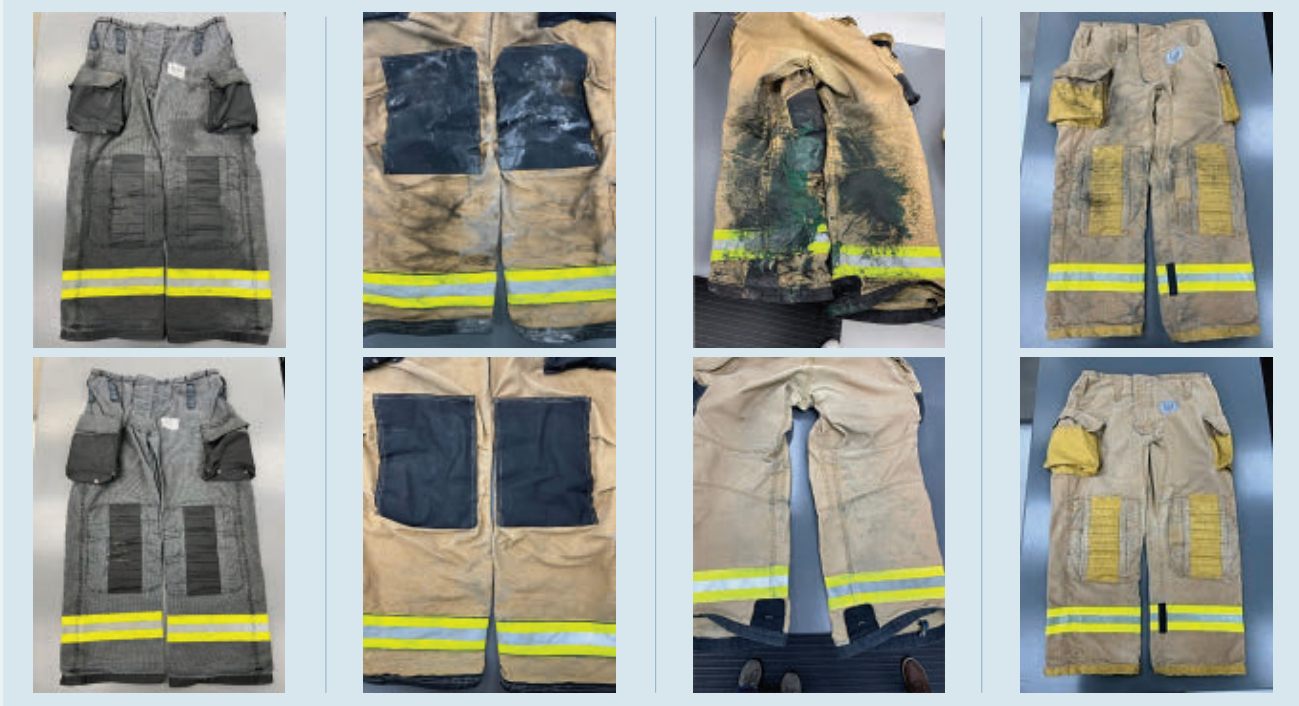
Figure E2. Evidence of Effective Residue Removal Using CO 2 + Cleaning System from CCT: Top—as Received, Bottom—After Processing
